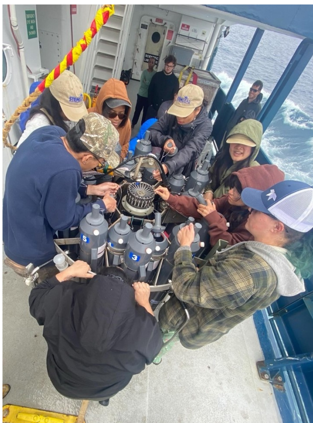
Students aboard the STEMSEAS R/V Atlantis did scientific research with a Conductivity, Temperature, Depth Sensor with Sampler Rosette.
